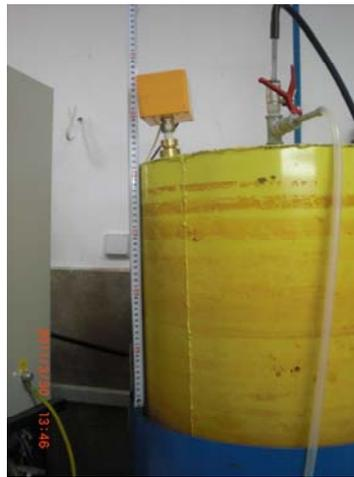
Fig. 6 Sensor for biogas flow rate
