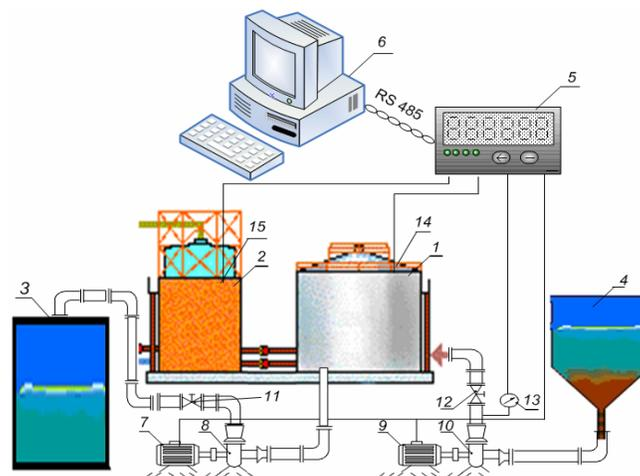
Fig. 1 Scheme of the pilot-scale biogas plant with a system for monitoring and control:
