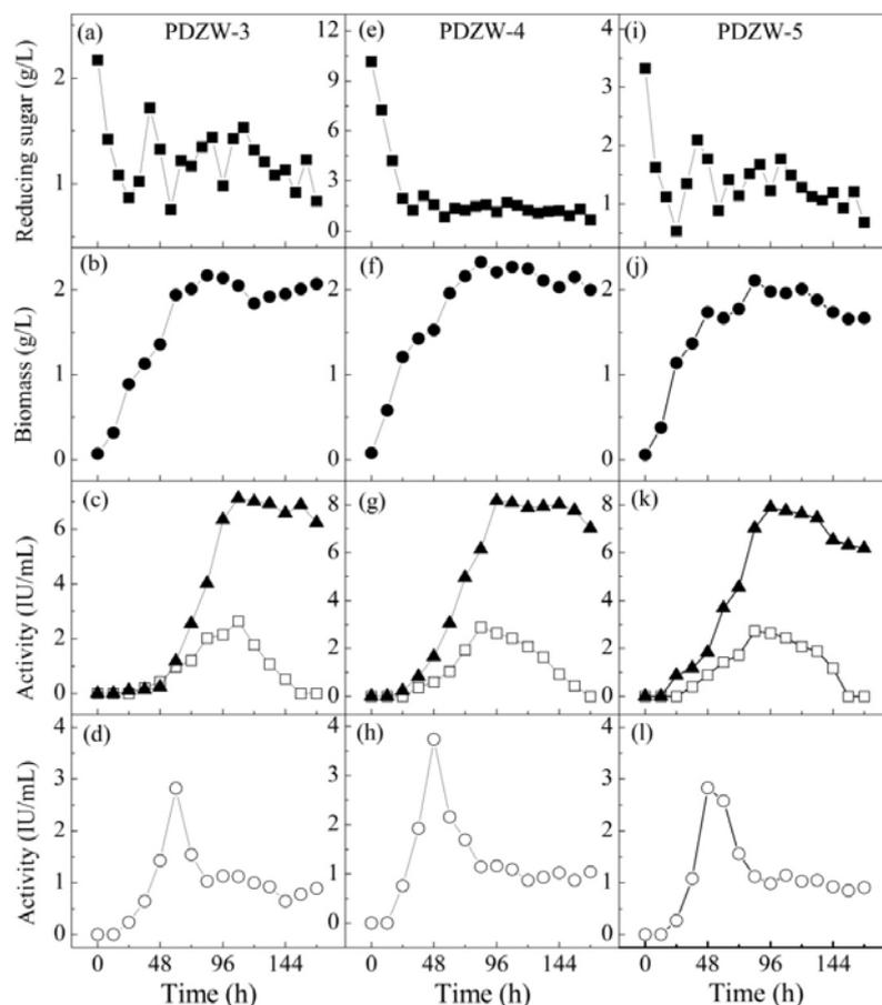
Fig. 4 Time course of reducing sugar (■), biomass (●),  $\alpha$ -rhamnase (□),  $\beta$ -glucosidase (▲) and amylase (○) in bioreactor cultivation of PDZW by *T. reesei* (a-d: PDZW3; e-h:PDZW4; i-l: PDZW5)
