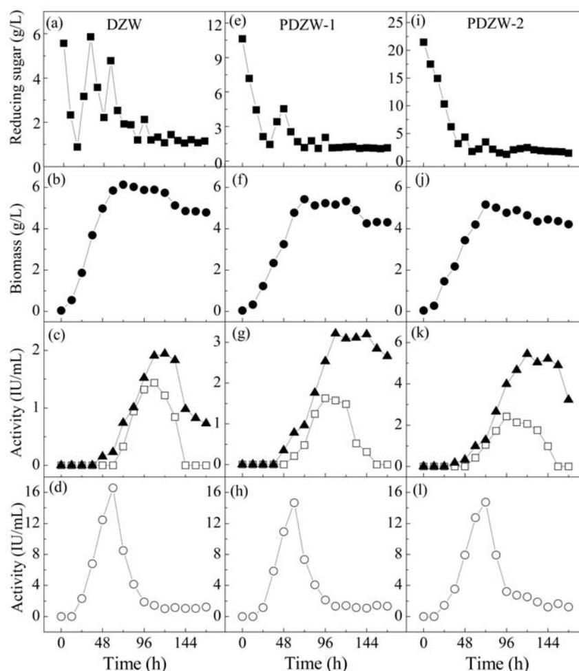
Fig. 3 Time course of reducing sugar (■), biomass (●),  $\alpha$ -rhamnase (□),  $\beta$ -glucosidase (▲) and amylase (○) in bioreactor cultivation of DZW and PDZW by *T. reesei* (a-d: DZW; e-h: PDZW1; i-l: PDZW2)
