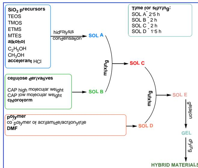
Fig. 2 Schematic illustration of hybrid membranes synthesis
