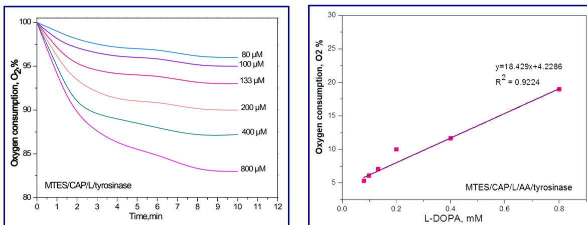
Fig. 4 Response time of the optical biosensor based on MTES/CAP/L/tyrosinase at different L-DOPA concentrations and calibration curve of L-DOPA
