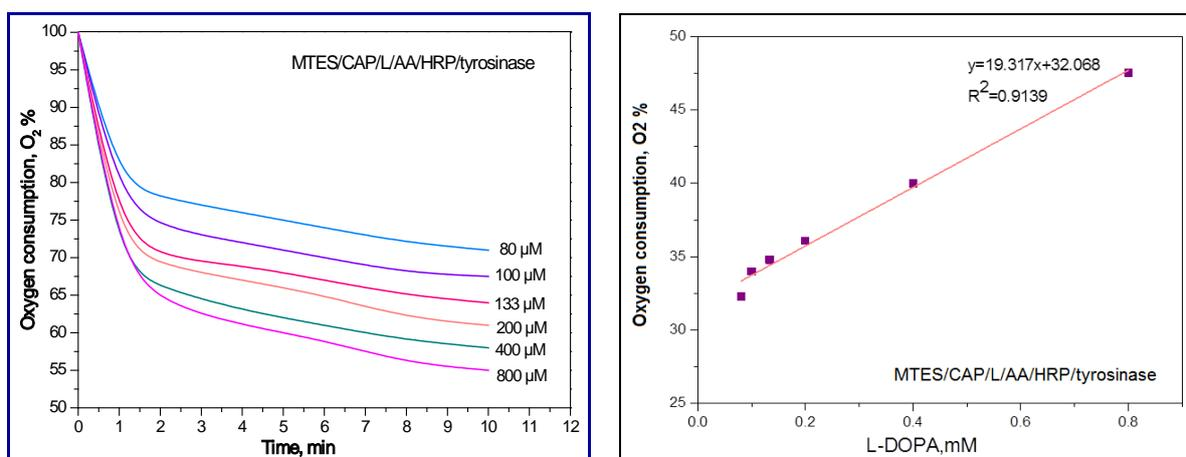
Fig. 5 Response time of the optical biosensor based on multi enzyme system at different L-DOPA concentrations and calibration curve of L-DOPA
