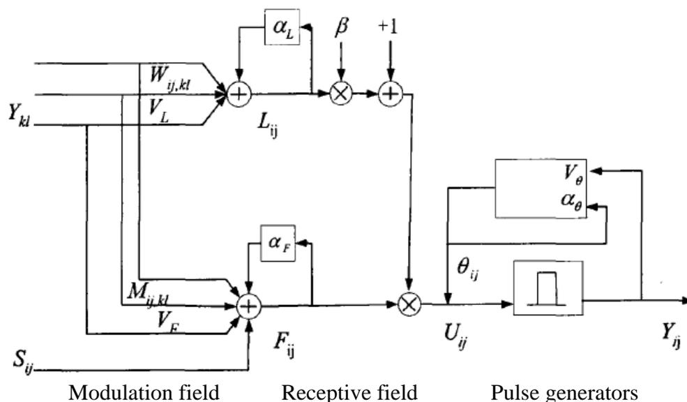
Fig. 1 The structure of traditional PCNN neuron
