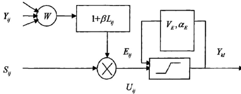
Fig. 2 Structure of the simplified PCNN neuron
