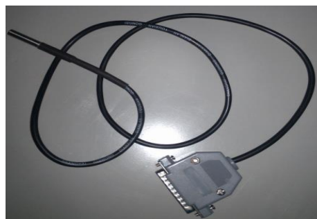
Fig. 2 Structure of LPT parallel pins interface Fig. 3 Image of temperature detecting module
