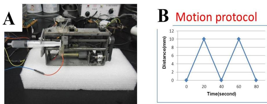
Fig. 2 (A) Picture of mechanical drive system (Picture of 5 ml plastic syringe with air combined with mechanical system); (B) Representative motion protocol.
