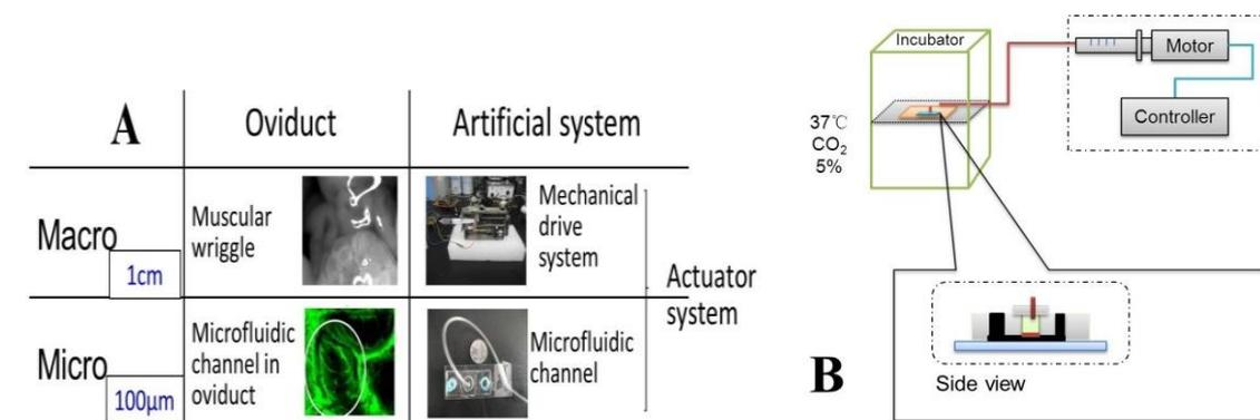
Fig. 1 (A) Summary of the oviduct and artificial system; (B) Schematic view of a system combining the mechanical drive system and PDMS microfluidic channel [8].
