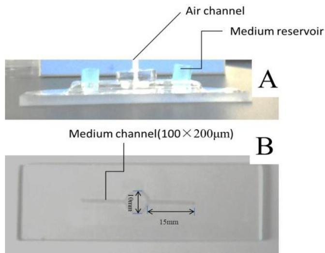
Fig. 3 (A) Side views of the PDMS microfluidic channel, respectively; (B) Presentation of the top view of the channel.
