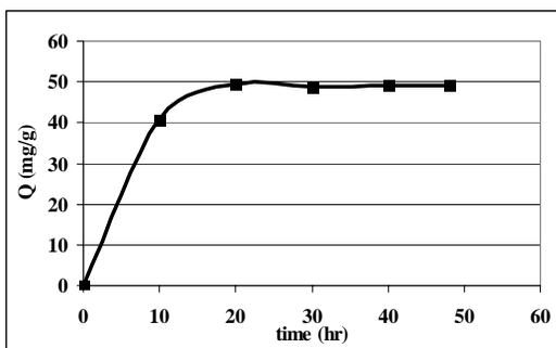
Fig. 3. Kinetic of adsorption of oxaliplatin by HAP (Q: amount of oxaliplatin adsorbed per 1 gram HAP)
