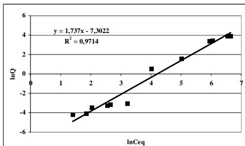
Fig. 2. Freundlich adsorption isotherm of oxaliplatin by HAP: natural logarithm of the amount of oxaliplatin adsorbed per gram HAP ( $\ln Q$ ) vs. natural logarithm of the oxaliplatin equilibrium concentration ( $\ln C_{eq}$ ). (Equilibration time: 48 hours)
