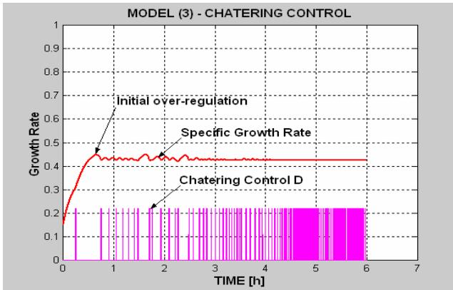
Fig. 1 Chattering control and stabilization of the specific growth rate
