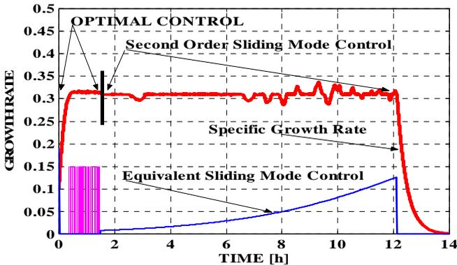
Fig. 2 Optimal profile and stabilization of the fed-batch process
