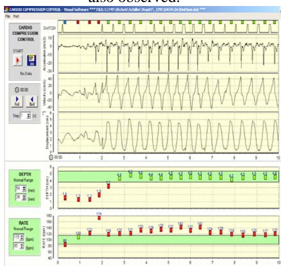
Fig. 9a The beginning of the CPR attempt of a volunteer. Start with: (i) incomplete recoil, corrected to perform recoil just after the 3 rd compression; (ii) smaller CC depth (1.5 cm), corrected to the normal levels (~ 4.5 cm) just after the 5 th compression; (iii) higher than the normal CC rate (118-142 cpm).
