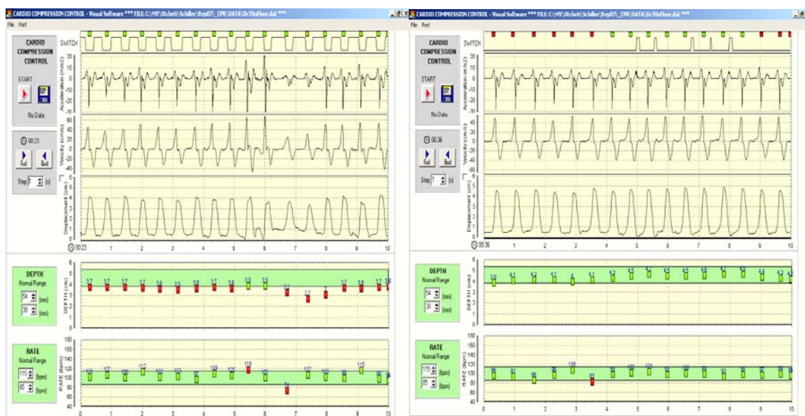
Fig. 11b After training, the same volunteer succeeds to provide CPR massage with correct CC rate and depth. The observed problems with the recoil are probably due to fatigue.
