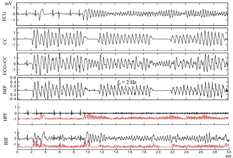
Fig. 7 Example of HPF and BSF filtering of VF mixed with CC (measured  $f_0 \approx 2\text{Hz}$ )
