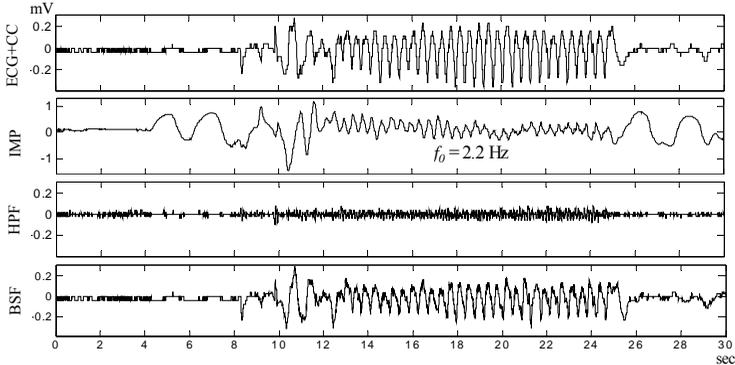
Fig. 9 Example of HPF and BSF filtering of real CC-contaminated ASYS. The fundamental frequency of the CC artefact is measured to be  $f_0 \approx 2.2\text{Hz}$
