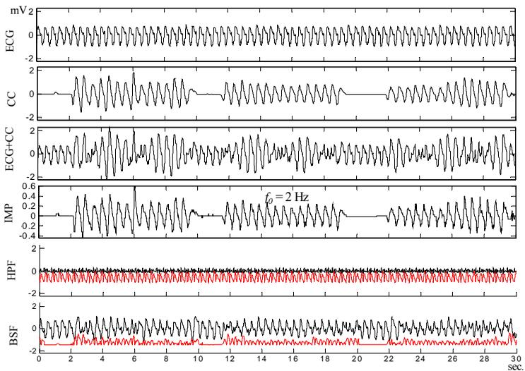
Fig. 6 Example of HPF and BSF filtering of slow VT mixed with CC (measured  $f_0 \approx 2\text{Hz}$ )
