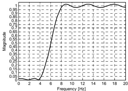
Fig. 2 Amplitude-frequency response of the designed filter HPF
