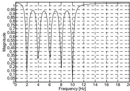
Fig. 3 Amplitude-frequency response of the filter BSF for  $f_0=2$  Hz
