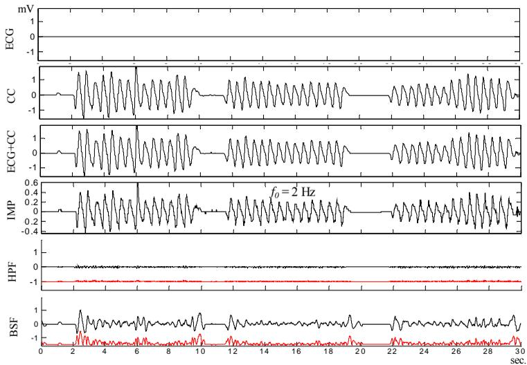
Fig. 5 Example of HPF and BSF filtering of ASYS mixed with CC (measured  $f_0 \approx 2\text{Hz}$ )
