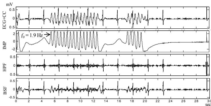
Fig. 8 Example of HPF and BSF filtering of real CC-contaminated NR. The fundamental frequency of the CC artefact is measured to be  $f_0 \approx 1.9\text{Hz}$
