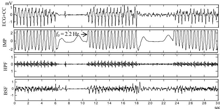
Fig. 10 Example of HPF and BSF filtering of real CC-contaminated ECG just at the moment of transition between NR and VF (between 12<sup>th</sup> and 18<sup>th</sup> second). The fundamental frequency of the CC artefact is measured to be  $f_0 \approx 2.2\text{Hz}$
