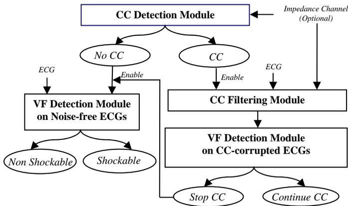
Fig. 1 Diagram of the shock advisory module in presence of CPR
