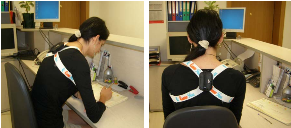
Fig. 1 Prototype of the technical device for prevention from spinal curvatures. Sound or vibration signal warns when trunk inclination forward or sideward is bigger than preliminary set angles by means of the position of build inside the plastic box 3 roll-ball tilt sensors from pendulum type.
