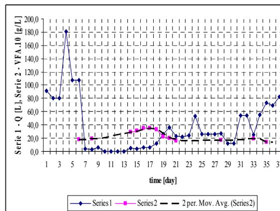
a) transient behaviour of  $Q$  (L) and VFA concentration ( $\times 10$  g/L)
