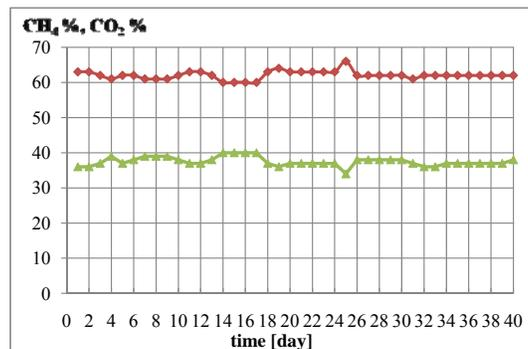
Fig. 15b Evaluations of CH<sub>4</sub> and CO<sub>2</sub> in the biogas during the experiment described in Table 1
