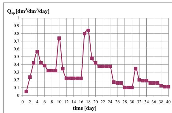
Fig. 15a Specific daily biogas flow rate evaluation during the experiment described in Table 1
