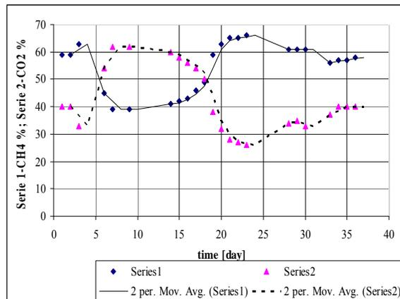
c) transient behaviour of CH<sub>4</sub> [%] and CO<sub>2</sub> [%]
