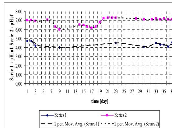
b) transient behaviour of pH of the influent and of the effluent
