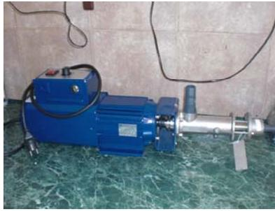
Fig. 5 Progressive cavity type pump
