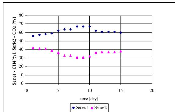
b) transient behaviour of CH<sub>4</sub> and CO<sub>2</sub> (in %/vol)
