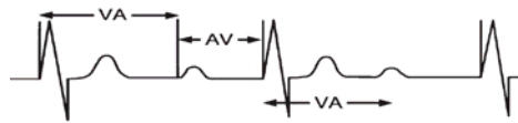
Fig. 9 DDI mode: the intrinsic atrial activity before the 3 rd QRS inhibits atrial pacing and the ventricles are paced after (VA + AV) period elapsed
