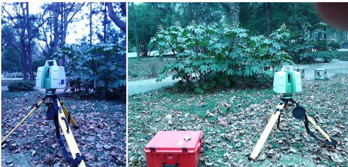
Fig. 1 Using Leica Scan Station C10 to scan trees on campus
