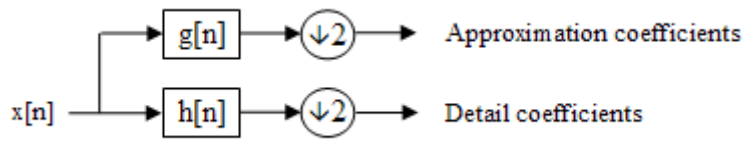
Fig. 4 Block diagram of filter analysis
