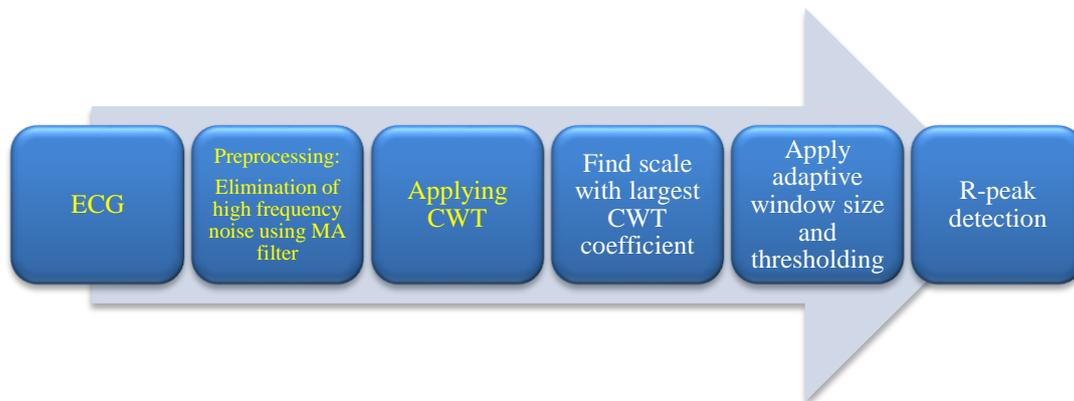
Fig. 3 A block diagram of the R-peak detection algorithm
