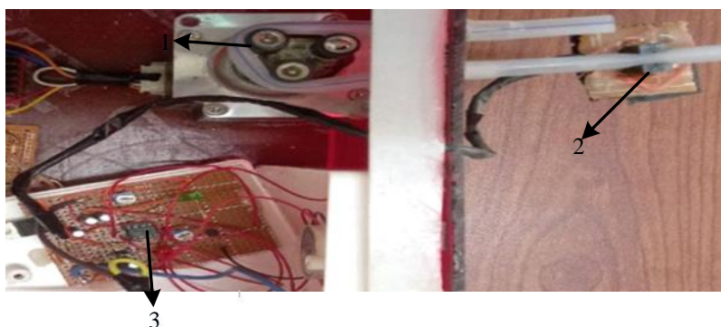
Fig. 3 Snap shot of the bubble detector circuit: 1 – Motor, 2 – Photo diode and photo transistor, and 3 – LM358 operation amplifier
